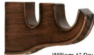
William 6" Double PO214WIDBK 1" W 3⅞" H backplate 7⅞" front return 3¼" back return Front cradle holds 2¼" diameter pole; back cradle holds 1⅝" diameter pole. Spicewood
