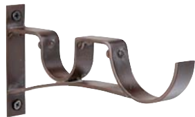
Harlan 6" Double PO200HADBK ¾" W 3¾" H backplate 6" front return 2¾" back return Front cradle holds 2" diameter pole; back cradle holds 1" diameter pole. Gossamer
